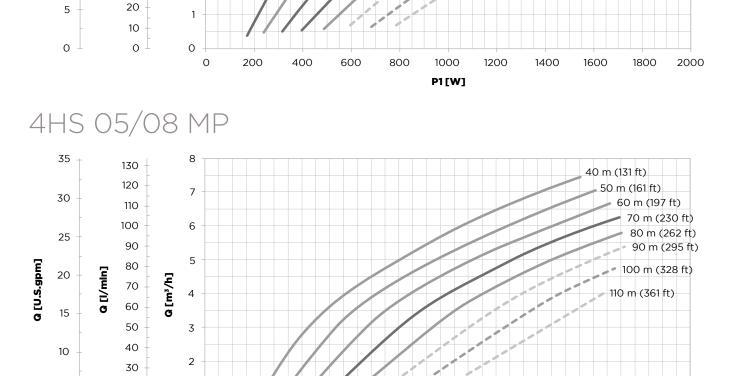
CM MultiPower installation is recommended for points of operation on the dashed lines.
