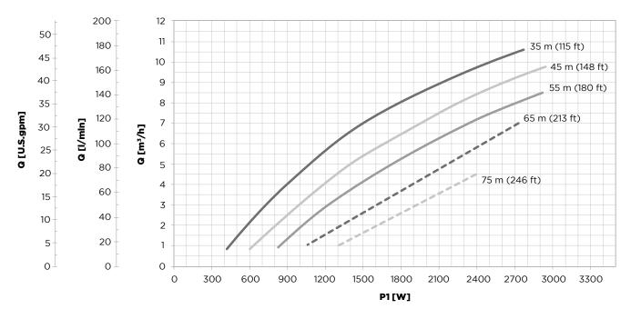
CM MultiPower installation is recommended for points of operation on the dashed lines.
